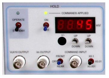
adjustment of the command potential. Two toggle switches directly below the COMMANDS APPLIED meter are used to step the applied command by  $\pm$  10 or  $\pm$  1 mV, respectively. A black push button is used to quickly swap the polarity of the applied holding potential. The maximum range for this control is  $\pm$  400 mV.
