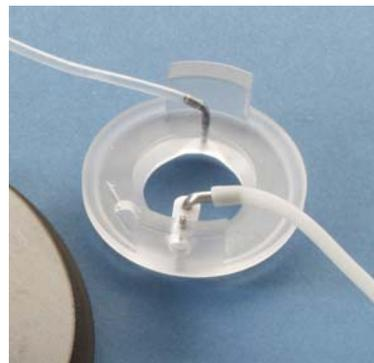
3. With the perfusion inlet tubing port directed towards you (i.e. roughly 6:00), slip the **RC-37** between the clips and into the clamped dish. The non-raised sections of the **RC-37** should easily slip under the clamps holding the dish. When properly installed, the white PTFE height adjusting component should be near the top of the clamped 35 mm dish (i.e. roughly 12:00).
