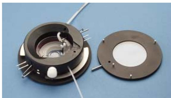
incubation system. Alignment is achieved via is via three metal posts and an alignment pin. The top section holds a 40 mm cover glass via a recessed annular lip and the cover glass is secured using a rubber o-ring. When in place, the cover glass seals a 36 mm widow useful for illumination purposes.
