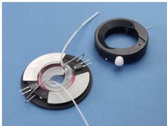
The small chrome tube shown in the picture above can be used to supply a slight vacuum to the chamber which will keep the top cover clear of condensation while the **DH-35i** is in use.
