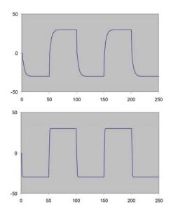
oscilloscope similar to that shown on the upper image. Adjust the CAP COMP control clockwise until the waveform on the oscilloscope is maximally compensated (see lower image). Overcompensation will induce instrument oscillation with loss of waveform and lighting of the INPUT OVERDRIVE LED.
