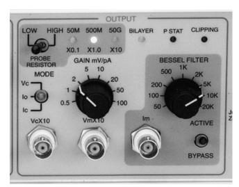
and **HB-205**, respectively). The *low* position is used for whole cell recording and selects the 500 M $\Omega$  resistor in the **LC-201** headstage and the 50 M $\Omega$  resistor in the **HC-202** headstage. It is not available in the **HB-205** headstage.
