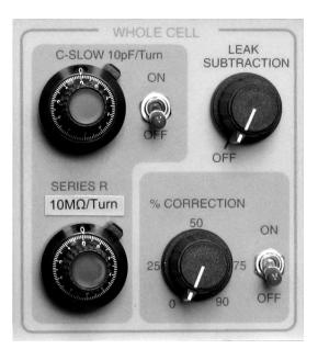
toggle switch disables C-SLOW allowing comparison with the uncompensated signal.
