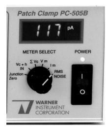
$V_m$ : This selection reports the transmembrane potential when in current clamp mode. Full scale range is  $\pm$  200 mV.
