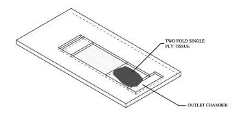
The upper wick should simply span the dam separating the bath chamber from the perfusion outflow chamber.
