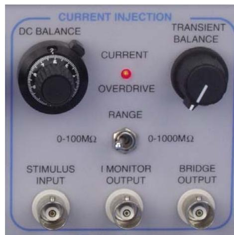
When balanced, the ten turn dial of the DC BALANCE control allows a reading of the electrode resistance. This reading is calibrated to the ELECTRODE RESISTANCE RANGE toggle.
