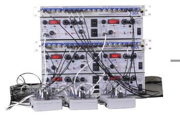
In the legacy USSING system, manual analog amplifiers were needed for experiment control.
